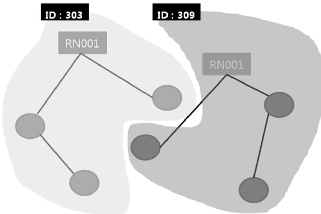
Wireless communication is not possible between devices that have the different network ID. Default network ID is 303. Radionode manager software is required for the devices to change network ID.
