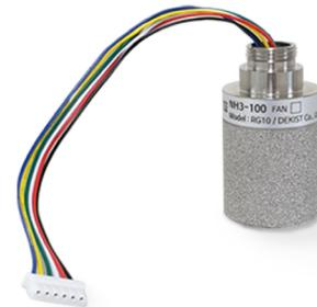
The RG10-NH3-100 is designed to be used with the RN400-T2GS model for measuring ammonia gas. It is a factory-calibrated gas sensor for which user calibration is not required at all. The entire unit would be replaced when the sensitivity degrades. An individual certificate is included in the product box. Using UA-Calibration software, the RN400-T2GS and a gas mixture, a professional customer could calibrate the RG10 at zero/span point.
