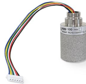
The RG10-H2S-50 is designed to be used with the RN400-T2GS model for measuring hydrogen sulfide gas. It is a factory-calibrated gas sensor for which user calibration is not required at all. The entire unit would be replaced when the sensitivity degrades. An individual certificate is included in the product box. Using UA-Calibration software, the RN400-T2GS and a gas mixture, a professional customer could calibrate the RG10 at zero/span point.
